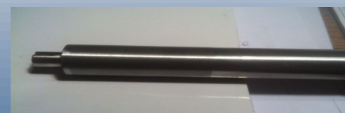
316 Stainless Steel Shaft with Tungsten Carbide coating sprayed and finished to original OD
