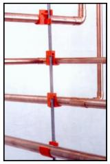
Place Hanger around rod as shown. Then twist until vertical and locked into place. Snap tubing into place.
