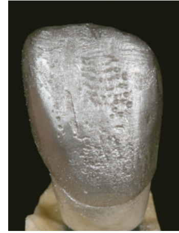
Fig. 7: : Application of silver powder to evaluate surface texture
